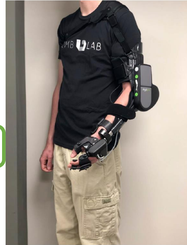
Figure 1. Patient with a left brachial plexus injury with inadequate elbow flexion with a MyoPro G device (Myomo, Inc, Cambridge, MA).
